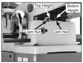
Figure 56. Infeed table positive stop bolts.
